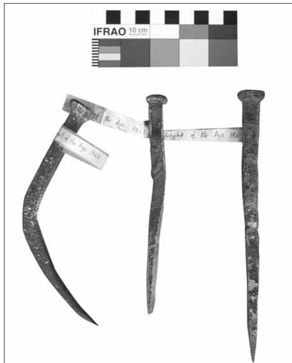
Fig. 4. Copper spikes from the Light of the Age (1858), privately held (Photo: J. Rodrigues).
