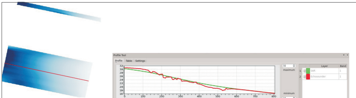
Fig. 10. Depth profiles from computed and echo-sounder maps in the selected area of Procida channel (depths are expressed in meters along y-axis).
