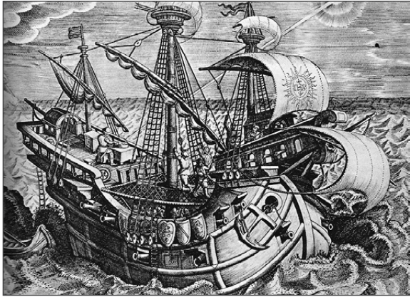
Fig. 41a. Anchor hanging from the starboard bow, with the crown swung aft (cited after J. Savant 1961, Histoire Mondiale de la Marine , p. 39).
