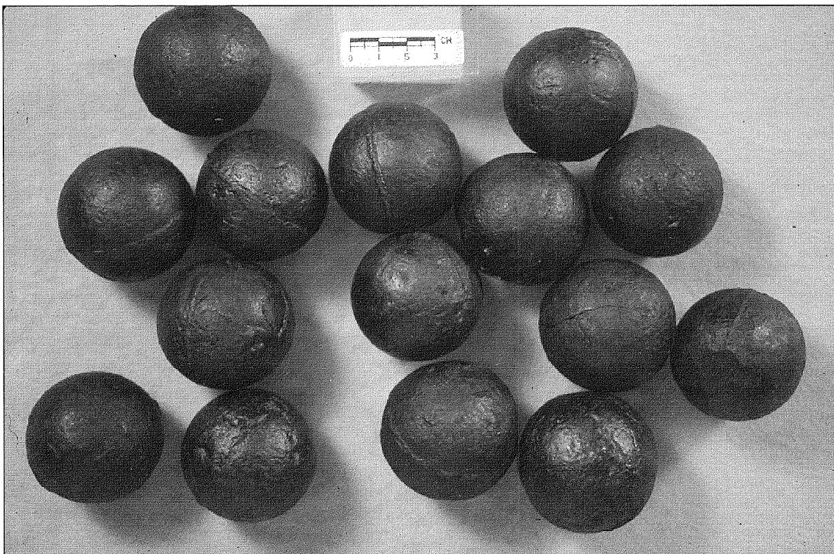
**Figure 7.** Cannon balls after conservation using electrolytic reduction.
