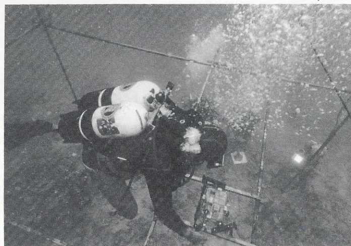
Fig. 2. Taking stereophotographs with the frame.
