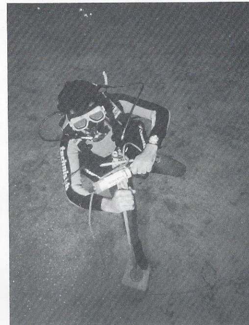
Fig. 2. Placing the SHARPS transmitter-receiver C in position.
